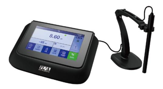
Suitable for high precision pH/conductivity measurements in scientific research, quality control, biotechnology and fine chemistry industry.
